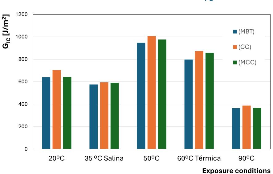
Critical energy release rate  $(G_{IC})$  calculated using the three formulations recommended by ASTM D5528:
