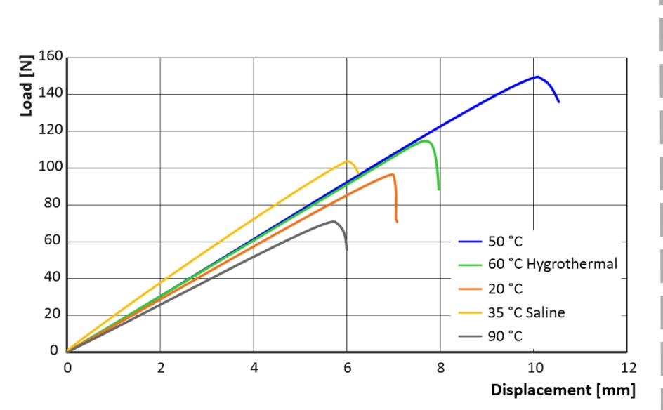
The curves display a similar initial slope, indicating that the stiffness of the adhesive joints remains almost unchanged for moderate temperature variations.
