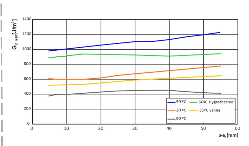
The evolution of the Mode I fracture energy with crack length also follows a temperature-dependent pattern.
